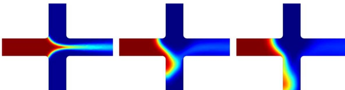
*Figure 6-11: The concentration distribution during the focusing (left) and injection stages (middle and right) in the electrokinetic valve's junction where the separation step is part of the injection stage. The graph of the separation step shows that there is incomplete detachment of the sample.*
