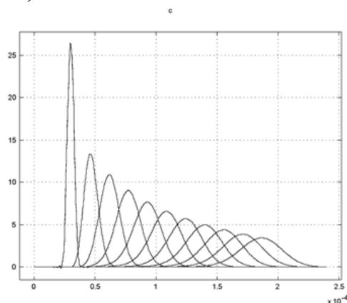
*Figure 6-14: Concentration profile along the length of the injection channel at different time steps: 0s, 0.06s, 0.12s, 0.18s, 0.24s, 0.3s, 0.36s, 0.42s, 0.48s, 0.54s, and 0.6s after initiation of the injection stage. The separation of the sample is substantially improved compared to the graphs in Figure 6-12.*
