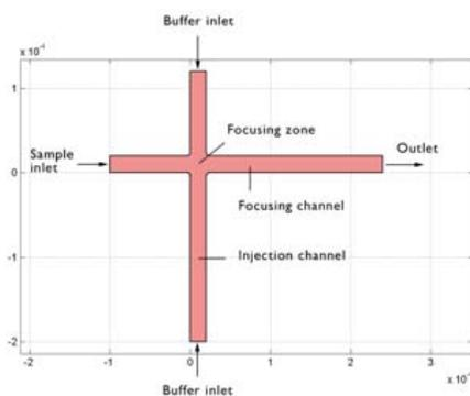
*Figure 6-9: The focusing stage involves pressure- and electro-driven flow of the sample and the buffering solution from the left, top, and bottom to the right. An electric field is then applied over the focusing zone to impose transport down through the injection channel.*
