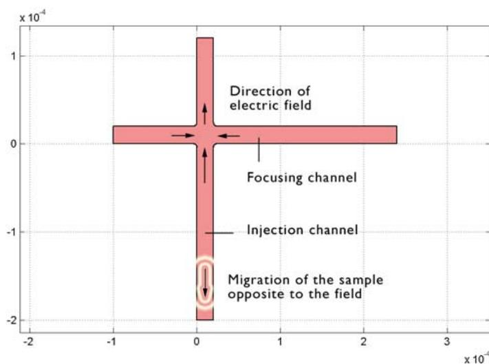
*Figure 6-10: During the injection stage, the convective flow is turned off and an electric field is applied. The horizontal field avoids the broadening of the sample while the vertical field injects the sample into the vertical channel in a direction opposite to the electric field.*
