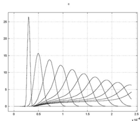
Figure 6-12: Concentration profile along the length of the injection channel at different time steps; 0s, 0.06s, 0.12s, 0.18s, 0.24s, 0.3s, 0.36s, 0.42s, 0.48s, 0.54s, and 0.6s after initiation of the injection stage. The incomplete detachment is clearly seen in the graph.
